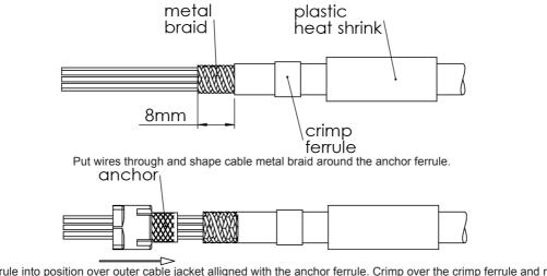
Slide the crimp ferrule into position over outer cable jacket alligned with the anchor ferrule. Crimp over the crimp ferrule and mount the D-Sub connector.
